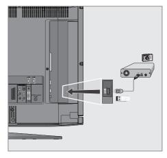
Connect the »USB« socket of the television and the corresponding socket on the data device (external hard drive, digital camera, card reader or MP3 player) using a USB cable;
